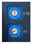
As shown in the figure, the high-level DIP switch (X16) set by the Profibus-DP address is dialed to 0, the DIP switch (X1) in the lower position is dialed to 3, this means that the address of the module in the DP network is set to 0\*16+3=3, and the valid address range of Profibus-DP is 1-125.
