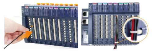
The module has a cable harness fixing end, which is used to fix the cable when the I/O module is connected to multiple cables.
