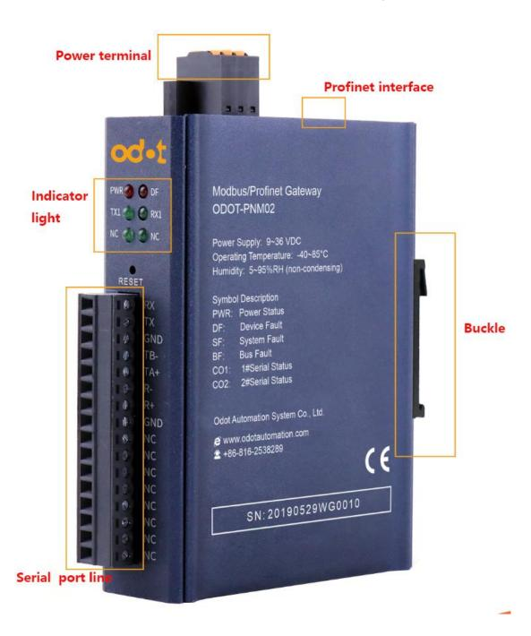
The upper panel has two ProfiNet interfaces and power connection terminals. PORT1 and PORT2, the two interfaces have the same function. These two interfaces have the switch function, that is, the host computer can access the equipment connected to PORT2 through the PORT1
