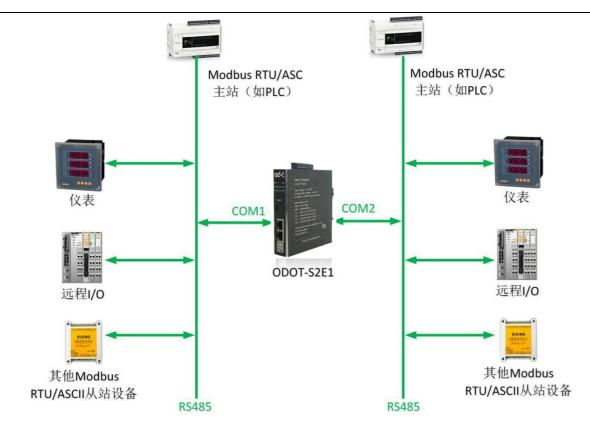
Figure 3.23 System topology diagram
