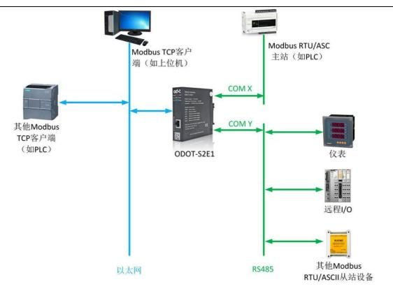
Figure 3.30 System topology diagram
