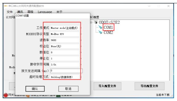
Figure 3.4 Set serial port properties
