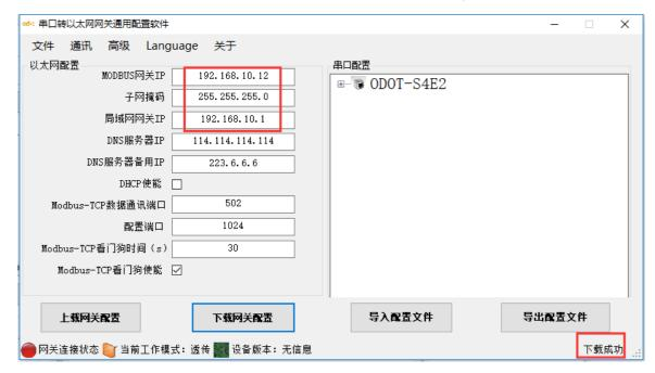
After the IP address is successfully modified, you need to change the computer's IP address to: 192.168.10.\* network segment.
