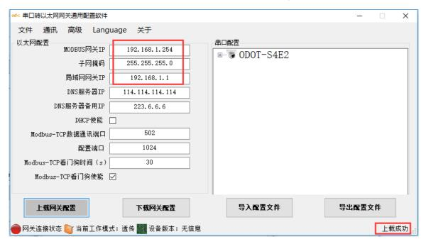
Modify the gateway IP address of the configuration software interface to: 192.168.10.12 (cross-network segment), and the LAN gateway IP to: 192.168.10.1. After the modification is completed, click to download the gateway configuration directly, and a warning box will pop up to confirm whether to modify the IP address. Click OK, you can see the download is successful in the lower right corner.
